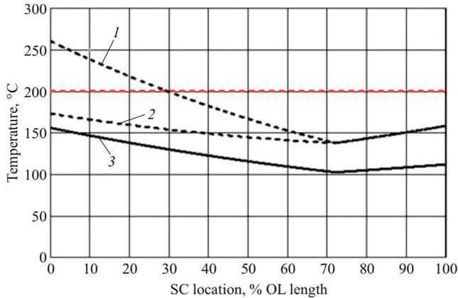
**Fig. 2.** Maximum calculated wire temperature of the 110 kV dual-fed OPTL as a function of SC location: 1, ACR failure; 2, ACR failure with reclosing from the side of a less powerful source; 3, no ACR.
