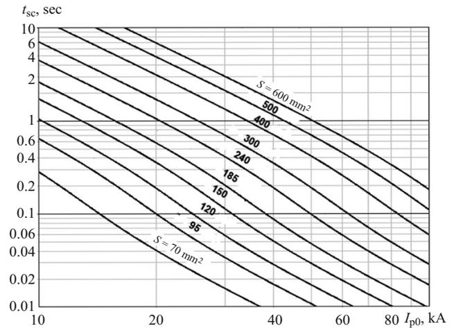
Fig. 1. Maximum allowable SC durations and currents based on thermal stability requirement for steel-aluminum wires.
